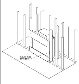
Figure 9.3 Proper Positioning, Leveling And Securing of an Appliance
